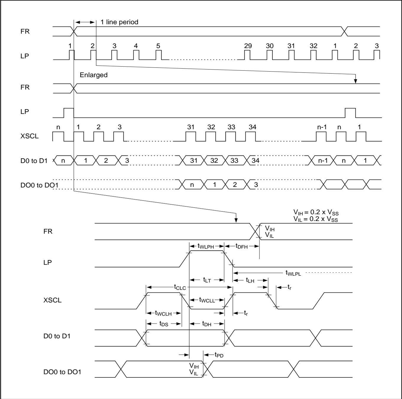
4.5 SEGMENT OUTPUT SIGNAL TIMING CHARACTERISTICS
