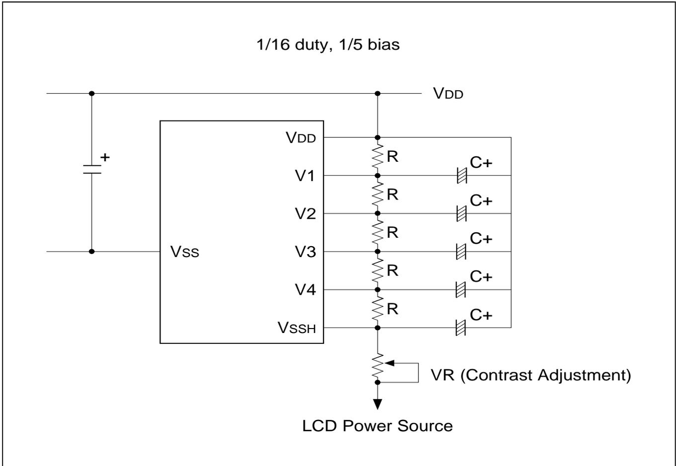
Note: Set the LCD power source conditions so that  $V_{SSH}$  does not exceed its maximum rating when  $V_R$  is short-circuited.
