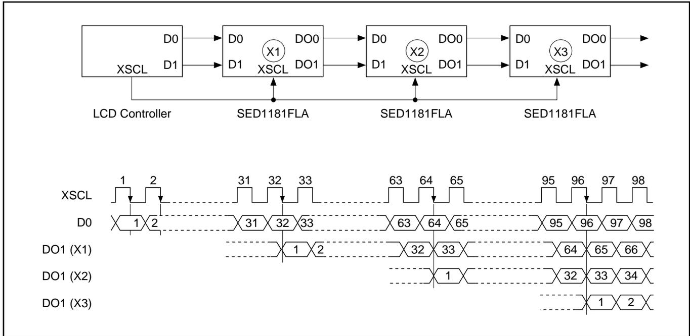
On the falling edge of the shift clock, XSCL, a one-bit shift right is performed. Segment display data at D0 and D1 is shifted into the LSB registers and the data residing in the MSB registers (which is apparent at DO0 and DO1) will be overwritten by the preceding register’s data.
