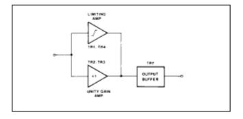
Fig.3 Block diagram
