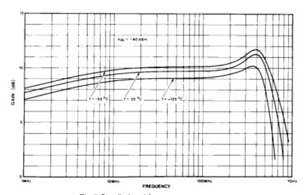
Fig.5 Small signal frequency response
