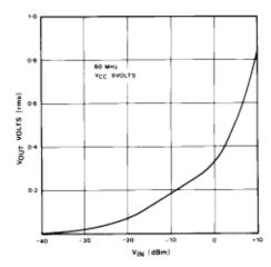
Fig.8 Transfer characteristics logarithmic input scale
