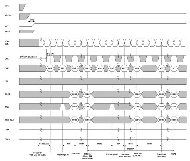
\* 200 cycle(tXSRD) of CK are required (for DLL locking) before Read Command
