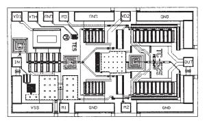
Chip Size: Chip Size Tolerance: Chip Thickness: Pad Dimensions: 1530 x 910 μm (60.2 x 35.8 mils) ±10 μm (±0.4 mils) 127 ± 15 μm (5.0 ± 0.6 mils) 75 x 75 μm (2.95 x 2.95 mils), or larger
