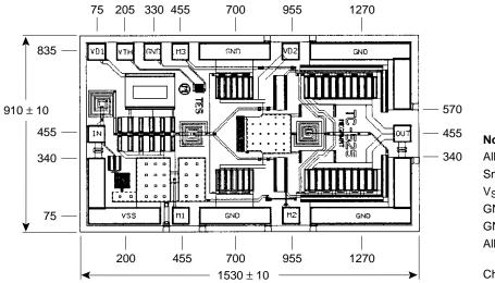
Figure 2. HMMC-5004 Bond Pad Locations.
