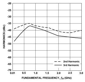
Figure 9. Typical Second and Third Harmonics vs. Fundamental Frequency at Pout = 21 dBm.
