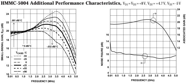
Figure 7. Typical Noise Figure Performance.
