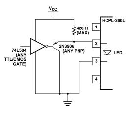
Figure 15. TTL interface circuit.
