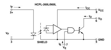
USE OF A 0.1 µF BYPASS CAPACITOR CONNECTED BETWEEN PINS 5 AND 8 IS RECOMMENDED (SEE NOTE 5).
