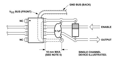
Figure 11. Recommended printed circuit board layout.
