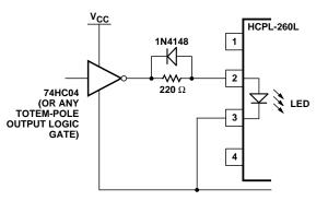
Figure 17. CMOS gate drive circuit.
