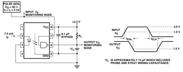
Figure 9. Test circuit for  $t_{EHL}$  and  $t_{ELH}$ .
