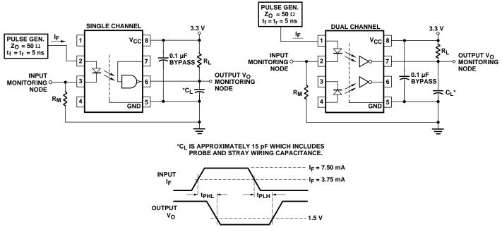
Figure 6. Test circuit for tPHL and tPLH.
