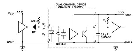
Figure 12. Recommended LVTTL interface circuit.
