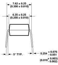
DIMENSIONS IN MILLIMETERS AND (INCHES). \*MARKING CODE LETTER FOR OPTION NUMBERS "L" = OPTION 020 "V" = OPTION 060 OPTION NUMBERS 300 AND 500 NOT MARKED.
