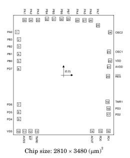
\* The IC substrate should be connected to VSS in the PCB layout artwork.
