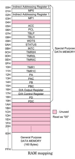
All data memory areas can execute arithmetic, logic, increment, decrement and rotate operations directly. Except for some dedicated bits, each bit in the data memory can be set and reset by the SET [m].i and CLR [m].i instructions, respectively. They are also indirectly accessible through Memory pointer registers (MP0;01H, MP1;03H).
