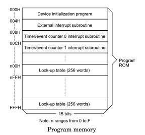
only. The TBLH is read only and cannot be restored. If the main routine and the ISR (Interrupt Service Routine) both employ the table read instruction, the contents of the TBLH in the main routine are likely to be changed by the table read instruction used in the ISR. Errors can occur. In other words, simultaneously using the table read instruction in the main routine and the ISR should be
