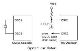
of a crystal, a resonator can also be connected between OSC1 and OSC2 to get a frequency reference, but two external capacitors in OSC1 and OSC2 are required.
