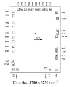
$\ast$  The IC substrate should be connected to VSS in the PCB layout artwork.
