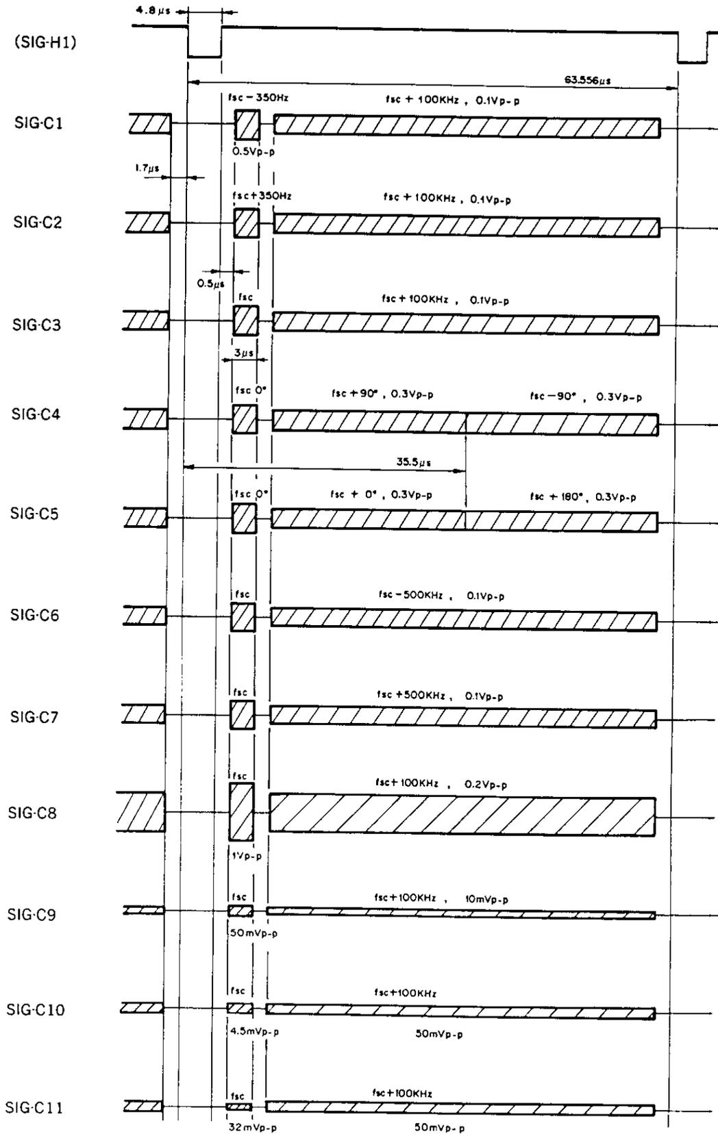
RGB system test signals
