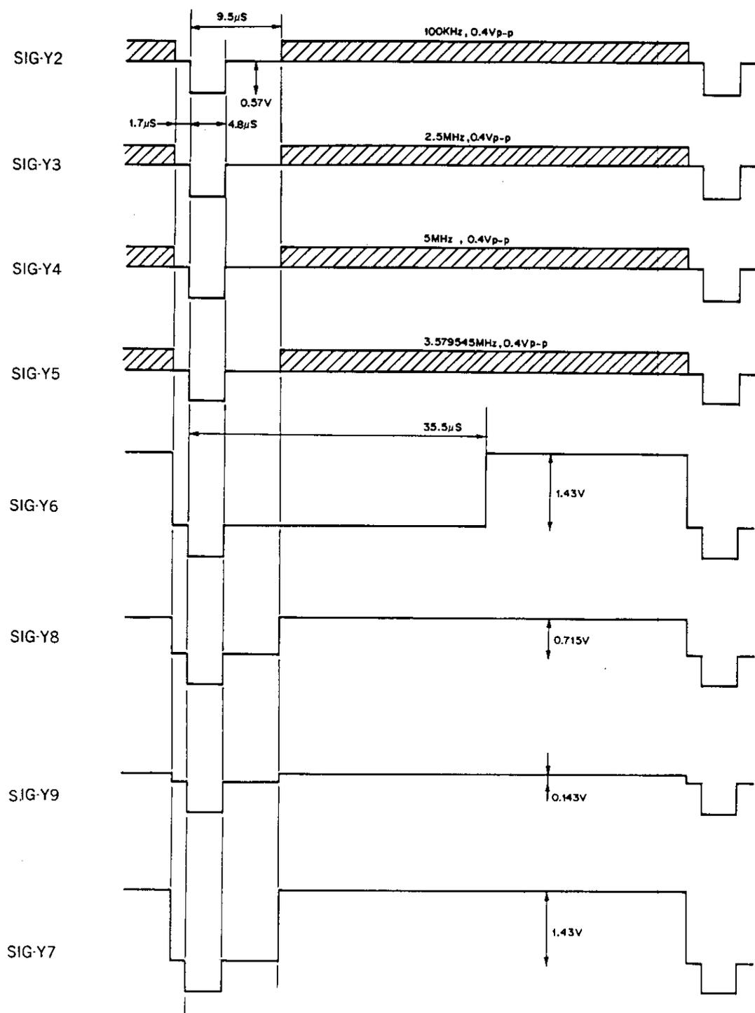
C system test signals  $f_{sc} = 3.579545\text{MHz}$
