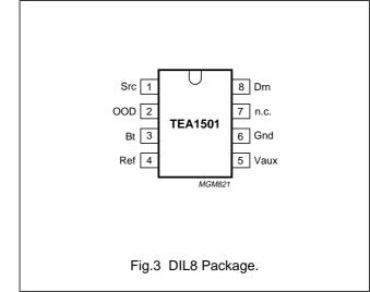
The TEA1501 contains a high voltage power switch, a high voltage startup circuit and low voltage control circuitry on the same IC. Together with a transformer and a few external components a low power, isolated, flyback converter can be built. The Greeny system operates in a burst mode. During each burst period the output voltage is regulated to a desired voltage level.
