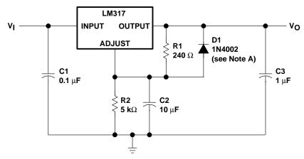
NOTE A: D1 discharges C2 if the output is shorted to ground.
