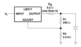
NOTE A: RS controls the output impedance of the charger.
