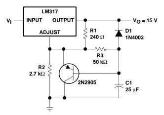
Figure 10. Slow-Turn-On 15-V Regulator Circuit
