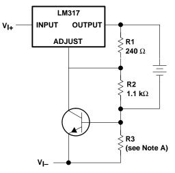
NOTE A: R3 sets the peak current (0.6 A for a 1- $\Omega$  resistor).
