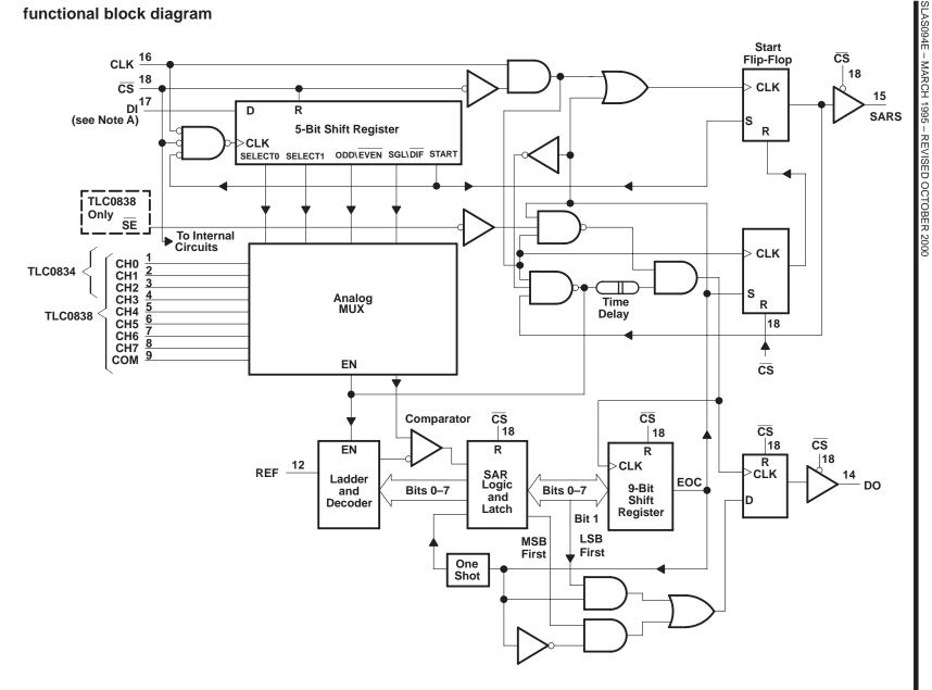
NOTES A: For the TLC0834, DI is input directly to the D input of SELECT1; SELECT0 is forced to a high. B: Terminal numbers shown are for the DW or N package.
