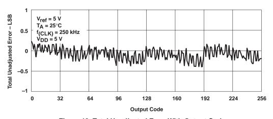
Figure 13. Total Unadjusted Error With Output Code
