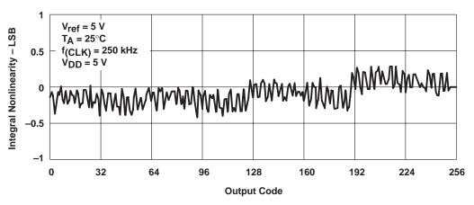
Figure 12. Integral Nonlinearity With Output Code
