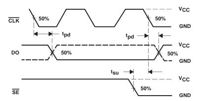
Figure 2. Data-Output Timing
